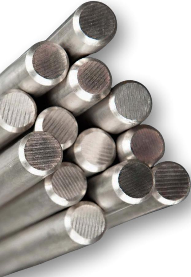
316LVM (Vacuum Melted 316L Stainless Steel) is a specially developed material for medical applications requiring high purity, biocompatibility, and corrosion resistance. The vacuum melting process enhances the material's homogeneity and purity, making it a reliable choice for implants and surgical instruments.
